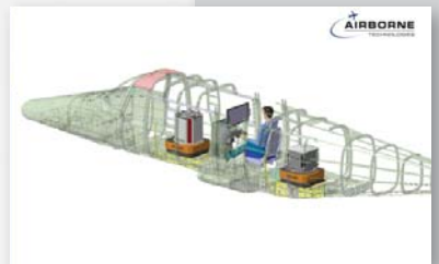
RIEGL LMS-Q1560 installed on GSM-3000 stabilized platform in the fixed-wing aircraft A-VIATOR AP68PT-600
