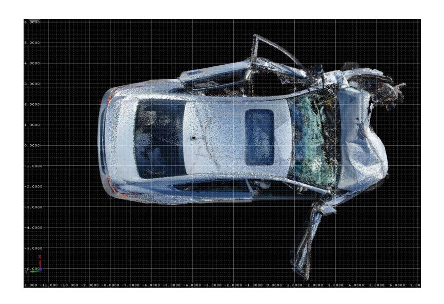
Scaled amplitude view in RiSolve indicates actual limit of intrusion for pole strike.
